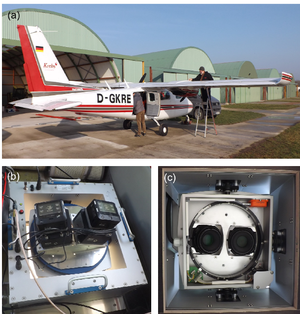
Figure 2. (a) Equipping a twin-engine aircraft for aerial digital surveys of marine wildlife, (b) View of a crosswise mounted tandem camera (PhaseOne IXA180) within a gyroscopically stabilized platform (GGs Speyer), (c) Exterior view of the camera system through the hatch of the aircraft
