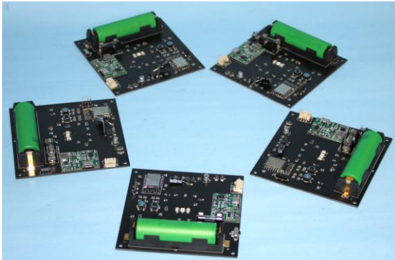
Figure 8. UV Targets developed for the calibration-procedure
