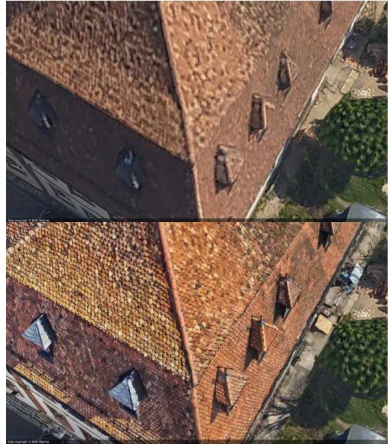
Figure 10 and 11: Details of the roof on the aerial model above at 5 cm GSD and the UAV model below at 0.5 cm GSD.
