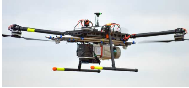
Figure 3: AeroSpector with Camera and Lidar combination
