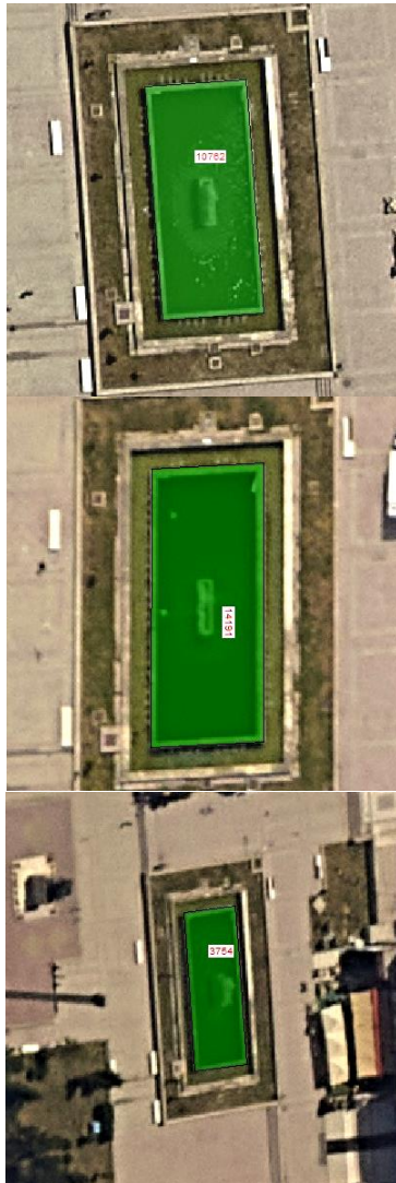
Figure 9. Up the target area measured in the nadir_3410 image, in the middle the higher resolution on image left_2955 and below the image right_3087 with the lowest resolution.
