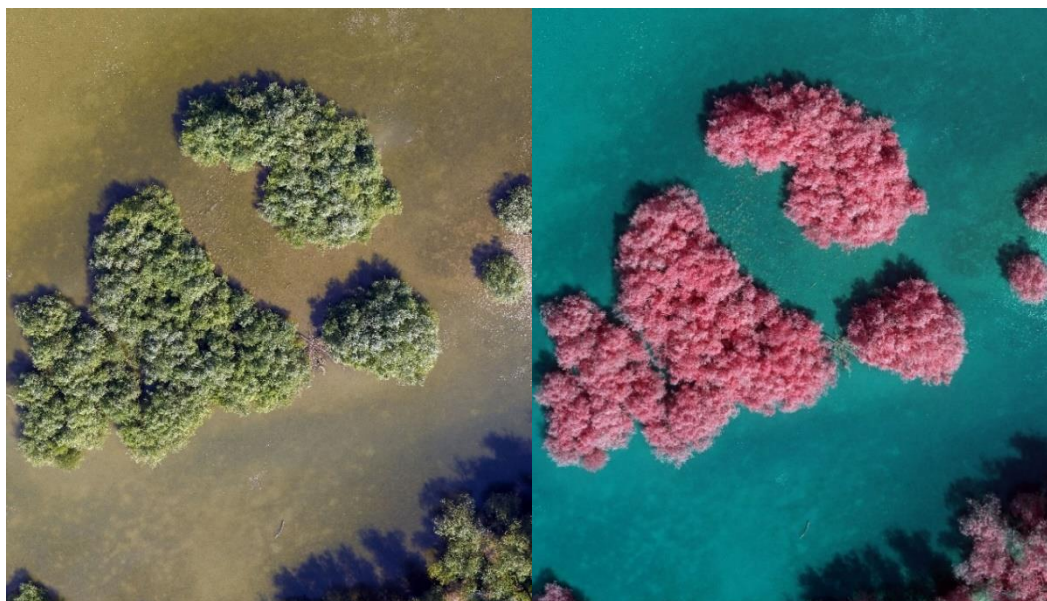
Figure 2. True Color Image of flooded area (left) and false-color composite (right) revealing chlorophyll
