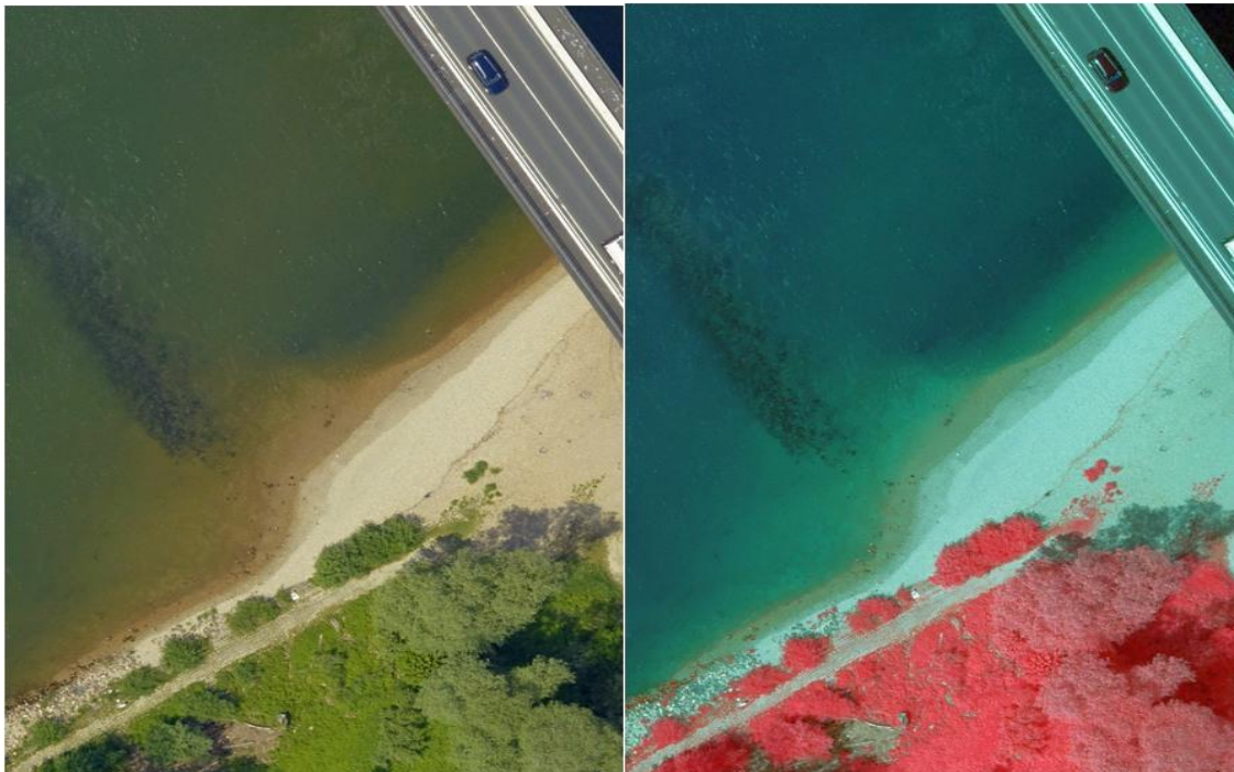
Figure 4. Comparison of True Color and NIR composite. The low chlorophyll content of the water shows there is a higher current which means the area is not a possible breeding ground for Aedes.
