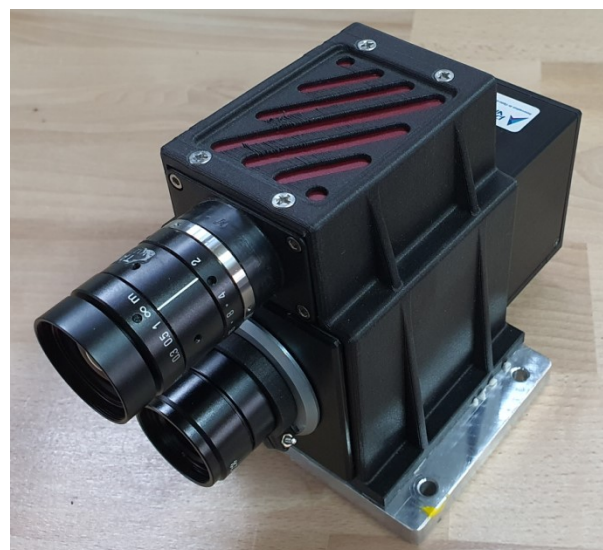
Figure 3. Corona camera consisting of daylight blind UV camera with a parallel RGB camera
