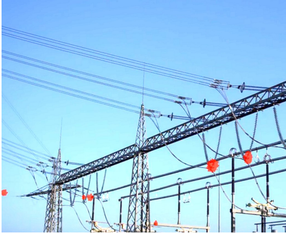
Figure 4: Result of a real time overlaid discharge detection of the UV Camera onto of the co-registered RGB Image
