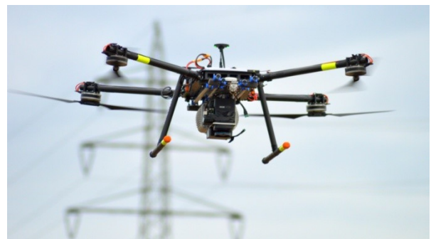
Figure 7: AeroSpector UAV at a mission with combined LiDAR and aerial imaging
