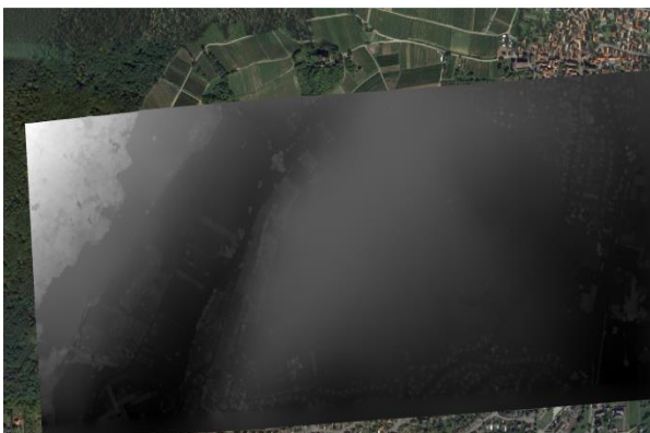
Figure 5. The DSM of the entire study area overlaid on the orthophoto.
