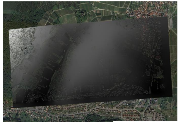
Figure 6. The DTM of the entire study with the cut off areas that represent buildings and higher vegetation. The grey values represent the DTM while all colored areas are from the orthophoto underlying this data set
