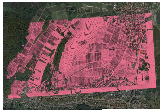
Figure 7. The final received vector based DTM with objects shown that are placed on top of the surface in colors from the orthophoto or the colored point cloud.
