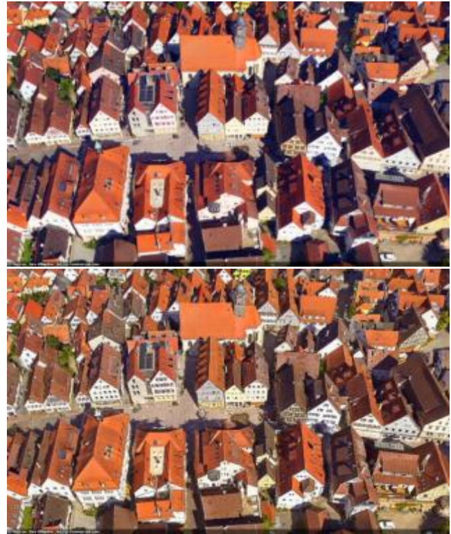
Figure 9-10 : Above: Marbach city centre generated using only oblique images; below: with the addition of the nadir camera
