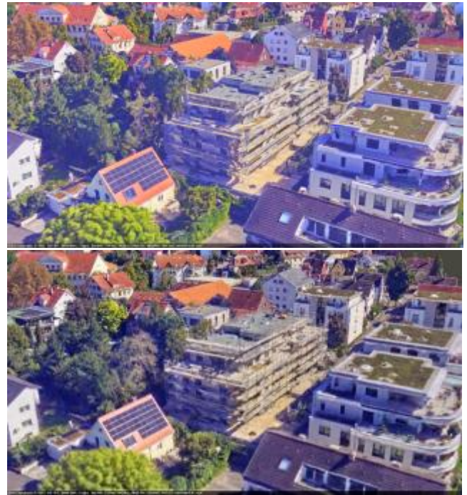
Figure 13-14 : Above: the result of normal processing; below: using Gaussian splatting from 8 perspectives
